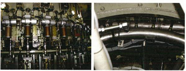
Bottle machine outfitted with air recovery system
